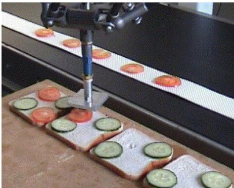
(a) Gripper mounted a manipulator.
