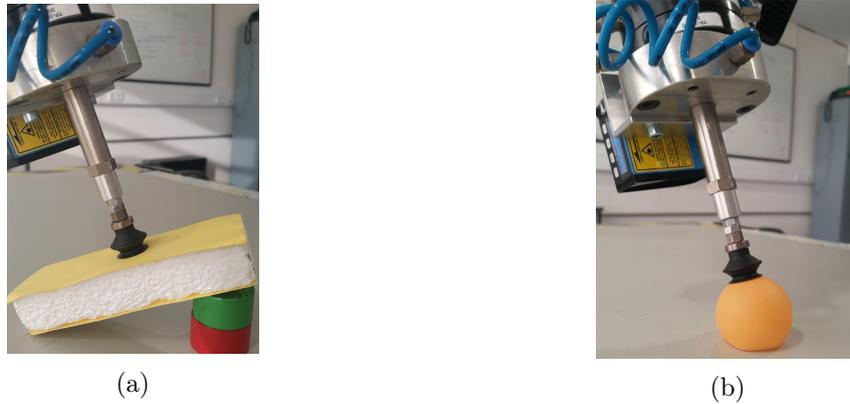
Figure 6.17: Gripper properly positioned to grasp different objects, one a flat surfaced object, (a), and the other a curved object, (b).
