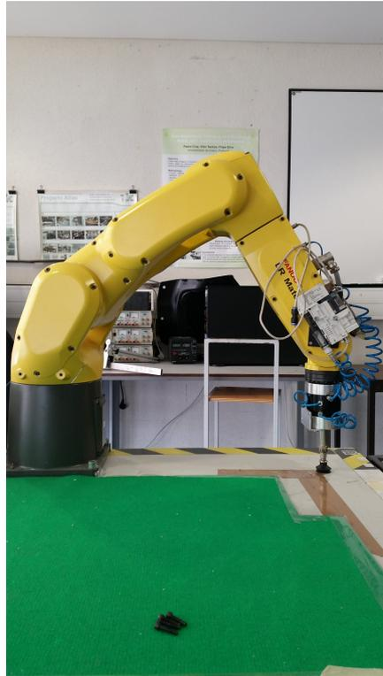
Figure 4.1: Robot's position for the end effector calibration.
