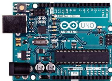
Figure 3.19: Arduino UNO board.
