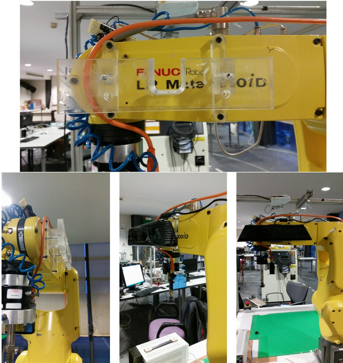
Figure 3.11: Kinect and Support fixed to the Robot.
