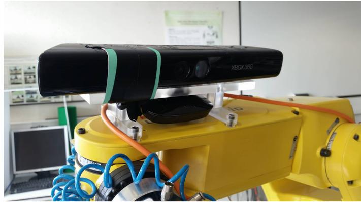
Figure 4.10: Kinect with the IR projector blocked for the intrinsic calibration of the IR (depth) camera.
