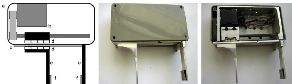
Figure 2.11: Gripper with force feedback for handling different types of fruits and vegetables [23].
